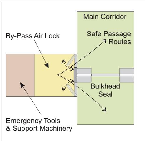
These lockers allow several people to move quickly and safely through from a damaged section into a safe one. This means a locker
