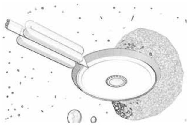
Such a tube can be constructed on Earth in one unit, packed for shipment and inflated into position in just a few hours. Compare that to the idea of assembling a pair of rigid structural rings over several weeks or months.
