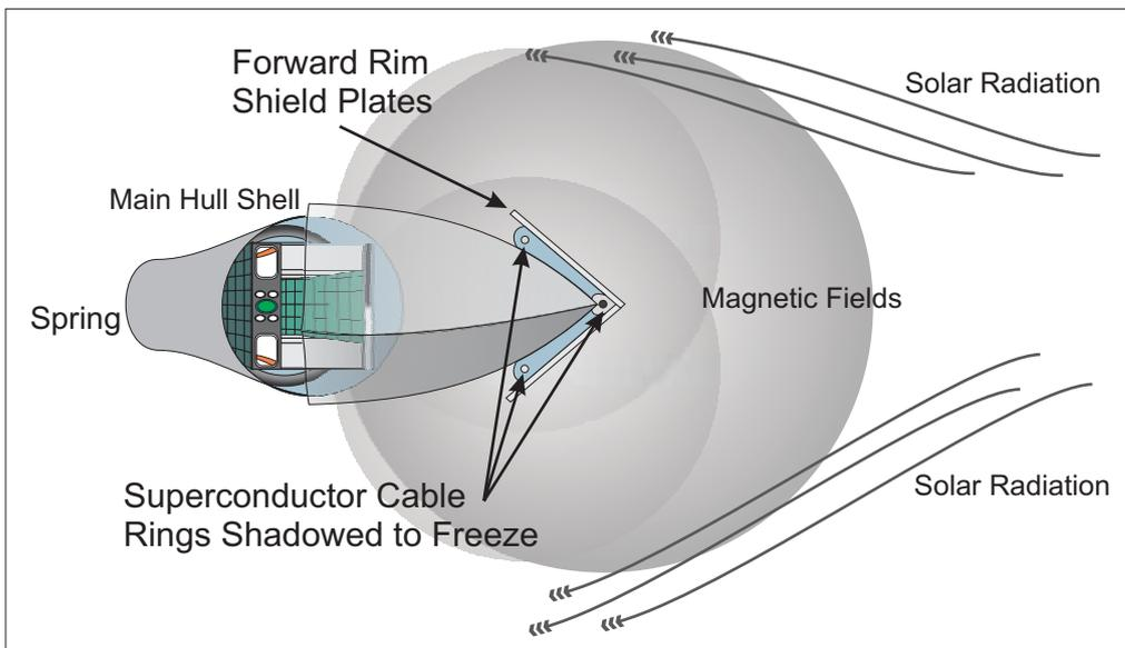
The problem with most superconductors is how to keep the coil for such a magnet cold; but in the shadows of space cold is easy to find.
