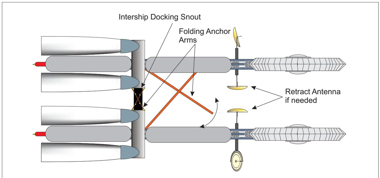
The entire assembly has a fail-safe break-away structure, to snap free if load becomes too great. This will prevent damage to the ships, crews, etc.
